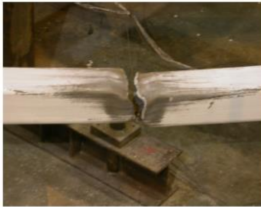
a) Fracture in the brace at 1.35% ODR
