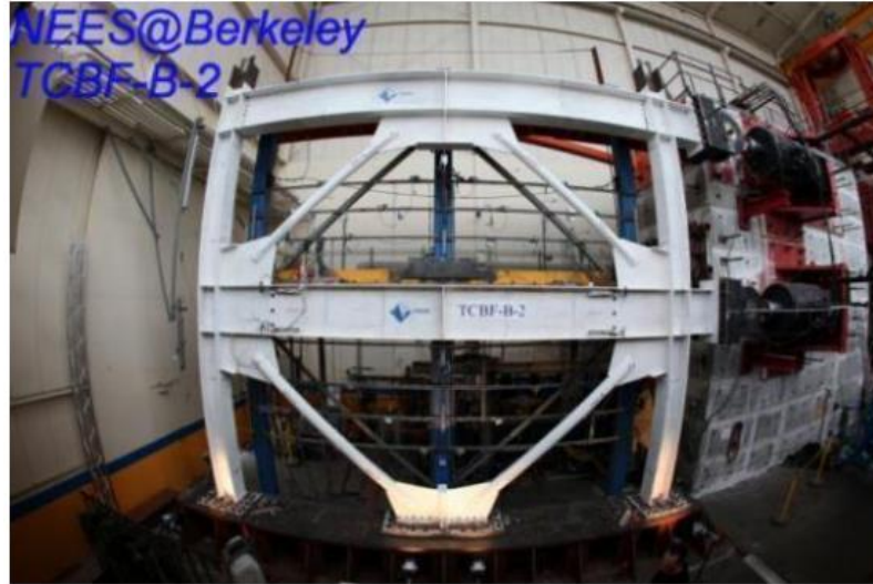
Figure 8: Test specimen constructed in UC-Berkeley by Lai and Mahin in 2013.
